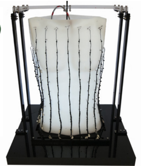
Simulated body-surface potential and a benchtop testing kit called a 'torso-tank', which is used to test the validity of the model.
